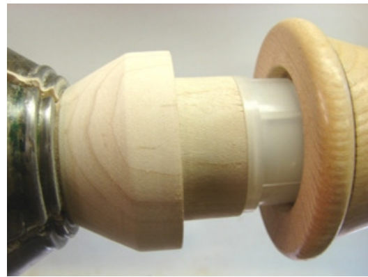
Fig 2 - bottom of mechanism ready to be pushed in
