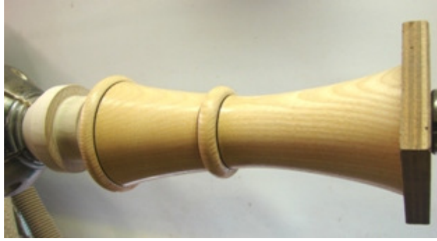
Fig 3 - CrushGrind shaft mechanism being pushed into the body of the mill
